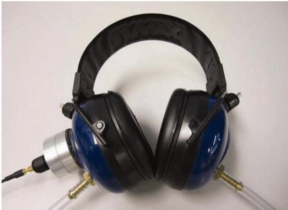
Figure 3. Complete acoustic headphones including twin 6 mm nozzles with attached tubing, microphone and occlusion ports (located on the cup either side of the head strap).
